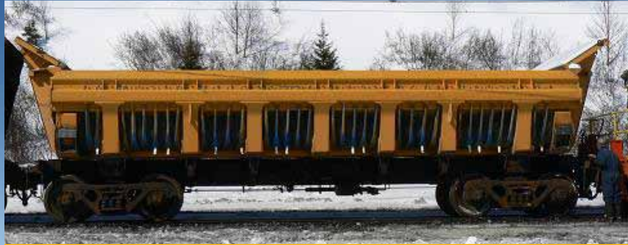
The Suspended Rubber System that Reduce Carry Back & Increase payload
